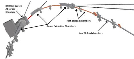
Figure 9: Conceptual layout of the arc sector vacuum chamber, photon extraction ports and absorbers.
