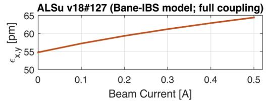
Figure 5: Emittance increase due to IBS as a function of current for nominal fill pattern, round beams, harmonic cavities, and a full set of undulators.
