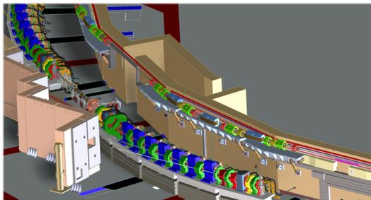
Figure 1: CAD model of ALS-U showing the existing accelerator tunnel with the new storage and accumulator rings.
