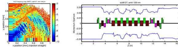
Figure 3: (Left) Frequency map for the 9BA baseline lattice with errors. (Right) Local momentum aperture for one period including errors.
