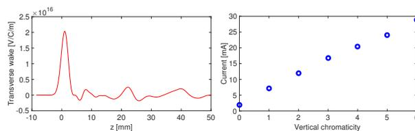
Figure 4: (Left) Total transverse wake function. (Right) TMCI threshold as a function of chromaticity.
