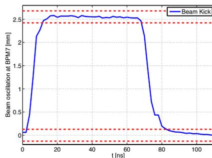
Figure 8: Beam integrated kick measured with turn-by-turn BPMs.
