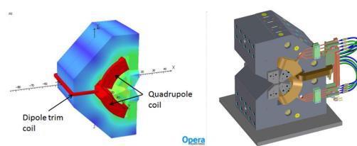
Figure 6: (Left) Field simulation for the transverse gradient dipole. (Right) CAD model of the R&D magnet which is being built to demonstrate the critical technical features of ALS-U magnets.
