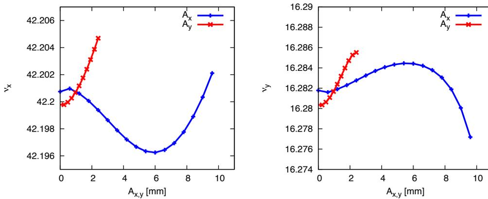
**Figure 3:** Amplitude-dependent tune shift in the MAX IV 3 GeV storage ring with octupoles at design strength.
