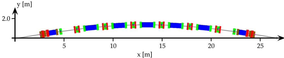
**Figure 1:** Schematic of one of the 20 achromats of the MAX IV 3 GeV storage ring. Magnets indicated are gradient dipoles (blue), focusing quadrupoles (red), sextupoles (green), and octupoles (brown).
