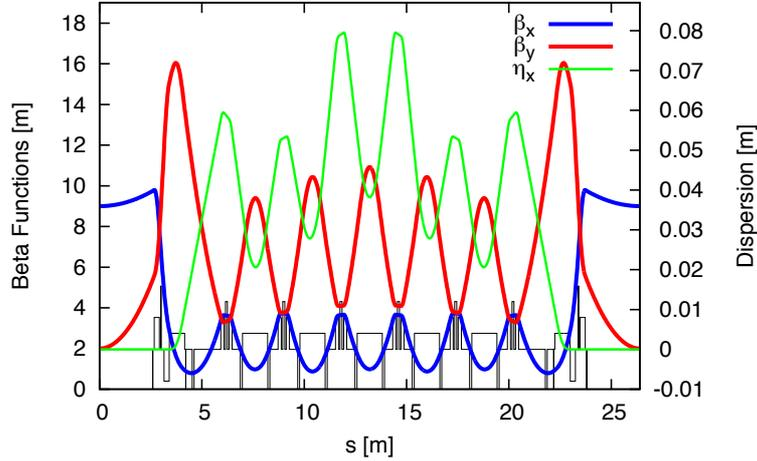
**Figure 2:** Beta functions and dispersion for one achromat of the MAX IV 3 GeV storage ring. Magnet positions are indicated at the bottom.
