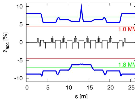
**Figure 7:** Momentum acceptance for one achromat of the MAX IV 3 GeV storage ring. A bare lattice and cavities at maximum voltage 1.8 MV have been assumed (green line, corresponds to 7% MA). For comparison, the red line shows 1.02 MV which corresponds to 4.5% MA in this configuration. The blue line shows overall MA, calculated from tracking with Tracy-3 for half a synchrotron period.
