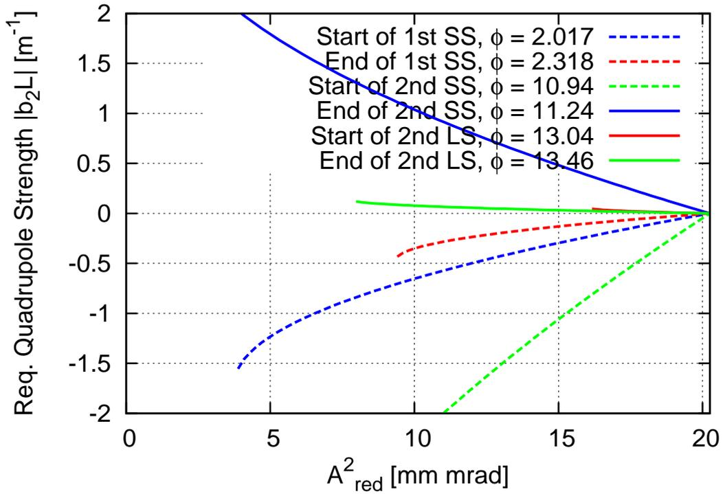
Figure 4: Field strength required from the pulsed quadrupole magnet in order to achieve a certain reduced invariant. Different locations in the lattice for the pulsed sextupole magnet are displayed. A quadrupole strength of  $(b_2L) \approx 1 \text{ m}^{-2}$  corresponds to the strongest quadrupoles used in the storage ring lattice.
