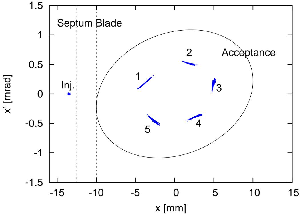
Figure 8: Injection with the PSM into the storage ring. Tracking data is shown at the injection point for injection and the first five turns in the storage ring. The blue dots are DIMAD tracking results for 1000 injected particles with  $\varepsilon_n = 1.5$  mm mrad,  $\sigma_\delta = 0.1\%$ , and a cut-off at  $3\sigma$ .
