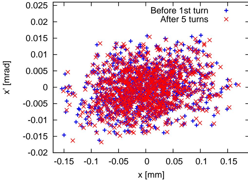
Figure 9: Effect of the PSM on the stored beam. The DIMAD tracking data shown here is taken at the location of the PSM with a cut-off at  $3\sigma$ . The blue + indicate stored beam particles before passage of the PSM. The red  $\times$  are tracking results for the same particles after the fifth turn. These particles received a kick from the PSM when it was pulsed during the first passage.
