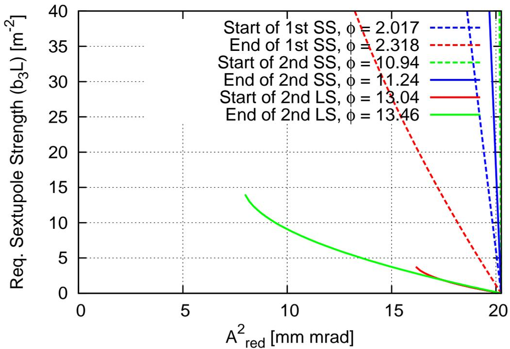
Figure 3: Field strength required from the pulsed sextupole magnet in order to achieve a certain reduced invariant. Different locations in the lattice for the pulsed sextupole magnet are displayed. A sextupole strength of  $(b_3L) \approx 21 \text{ m}^{-2}$  corresponds to the strongest sextupoles used in the storage ring lattice.
