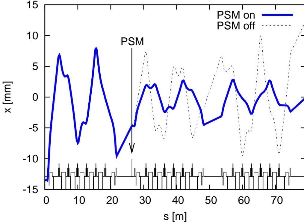
Figure 6: Orbit of the Injected bunch starting at the injection point further on through the PSM up to then end of the 4th LS. The dashed line indicates the orbit of the injected bunch if the PSM is turned off. Without the PSM the injected bunch will eventually hit the aperture as can be seen at the end of the 4th LS.
