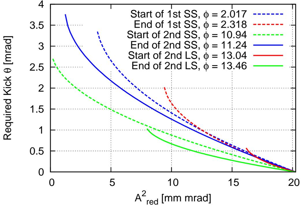
Figure 2: Kicks required from the pulsed magnet in order to achieve a certain reduced invariant. Different locations in the lattice for the pulsed magnet are displayed along with their phase advance with respect to the symmetry point.
