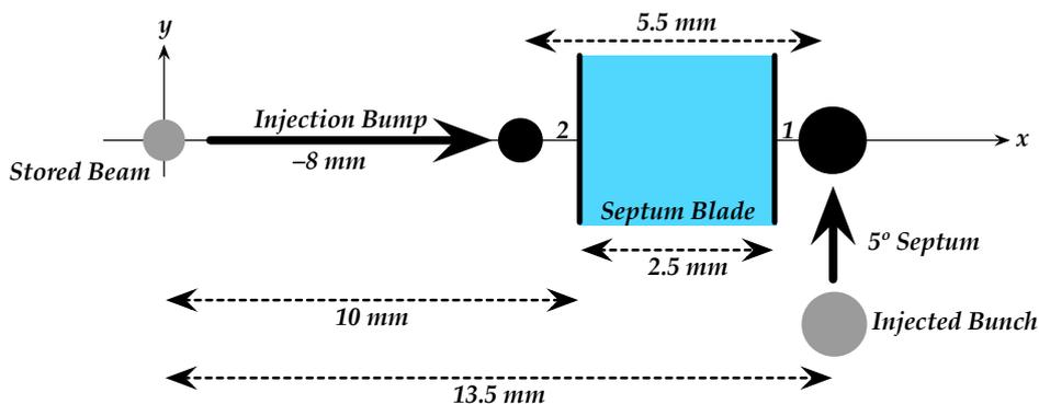
Figure 1: Schematic of the conventional injection scheme for the MAX IV 3 GeV storage ring as detailed in [3].
