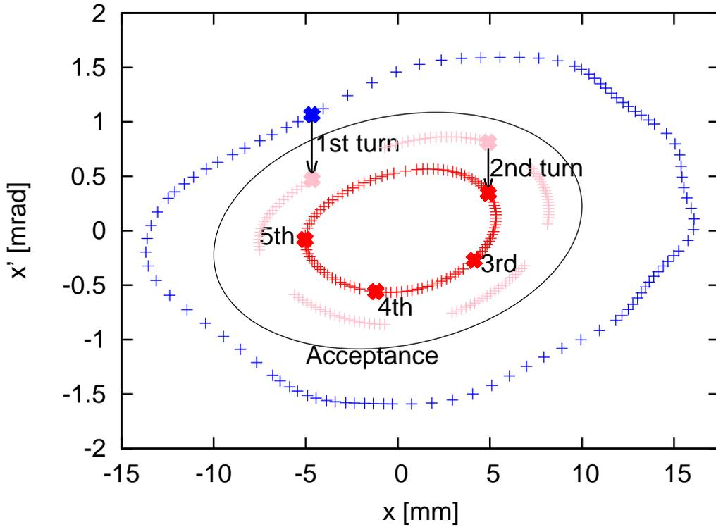
Figure 10: Two-turn injection with the PSM into the storage ring. Tracking data is shown for capture at the PSM (blue  $\times$ ) and for the first 100 turns in the storage ring (red  $+$ ). The outer “ellipse” (blue  $+$ ) is distorted due to the nonlinearities of betatron motion at large amplitudes (strong sextupoles!). The inner ellipse corresponds to more linear motion at the reduced invariant  $A_{\text{red}}^2 \approx 3.1 \text{ mm mrad}$ .
