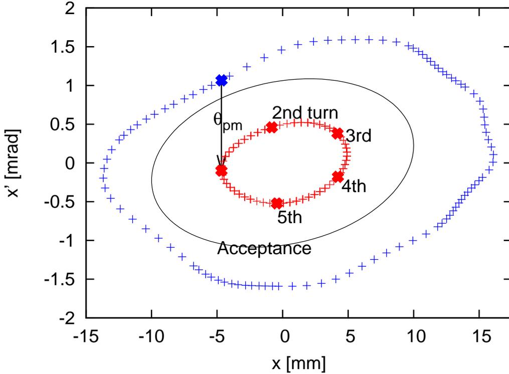
Figure 7: Injection with the PSM into the storage ring. Tracking data is shown for capture at the PSM (blue  $\times$ ) and for the first 100 turns in the storage ring (red  $+$ ). The outer “ellipse” (blue  $+$ ) is distorted due to the nonlinearities of betatron motion at large amplitudes (strong sextupoles!). The inner ellipse corresponds to more linear motion at the reduced invariant  $A_{\text{red}}^2 \approx 2.3 \text{ mm mrad}$ .
