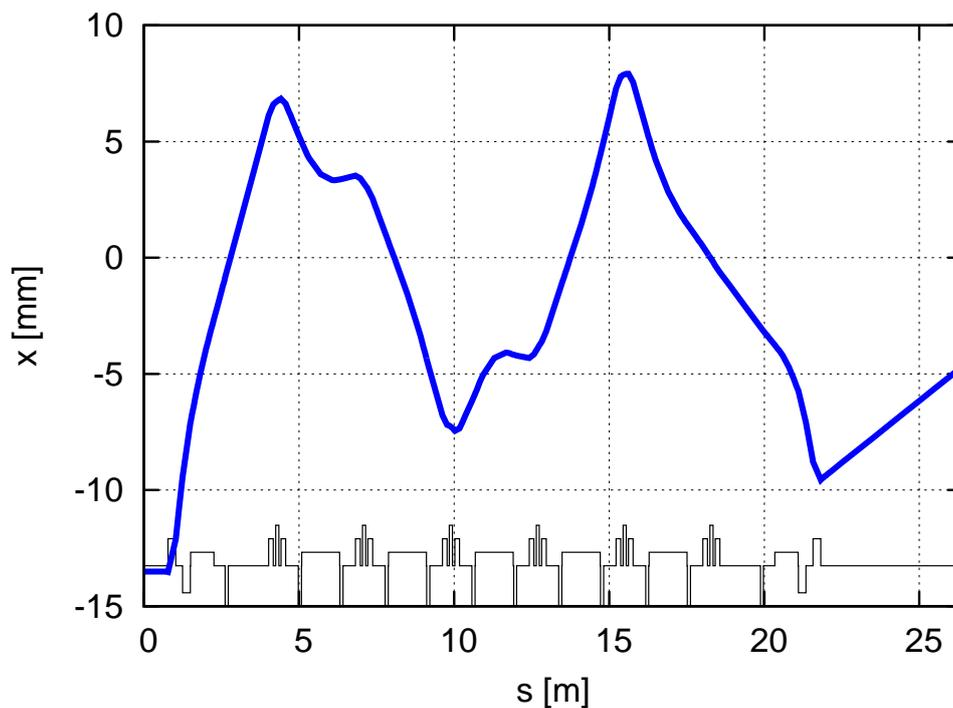
Figure 5: Orbit of the Injected bunch starting at the injection point and ending at the location of the PSM in the 2nd LS.
